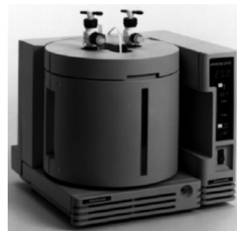
ATCS with 1500cc patented breakseal quartz bubbler.
