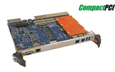
Diversified Technology's CPB4811 PICMG® 2.16-compliant packet switched backplane (PSB) processor blade combines high performance with low power for telecom and Internet IP-based applications.
