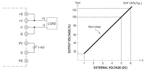
Note: (1)Reference voltage terminal, PS and PV are connected when shipping (2)+S & +V, -S & -V also need to be connected on CN1 or CN2.
