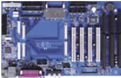
ETX-DB-7SR Full Function ETX Baseboard with LCD/CRT VGA, Audio, DOC, CF II & D I/O
