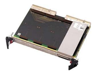
The D203 is a 6U M-Module carrier board for universal I/O on the CompactPCI bus as well as on PXI for automated testing requirements. It allows high flexibility in applications such as data acquisition or process control. The D203 supports all eight PXI trigger lines as defined in the PXI specification. You can install up to four M-Modules on the D203, which needs only one slot on the CompactPCI bus or
