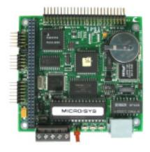
Netsock/100 provides a turnkey, network-oriented platform on which to build embedded systems. Based on the Micro/sys SBC1190 embedded PC and it's built-in 10BASE-T Ethernet port, Netsock/100 is a small PC/104 format computer that offers mid-range performances, and that can significantly reduce development time.
