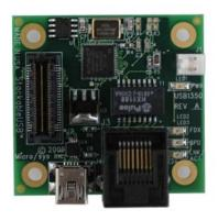
The USB1350 provides 10/100 Ethernet connectivity to any systems with USB. It is ideal for adding Ethernet ports to a system or upgrading Ethernet performance in older systems. Interfacing through a High-Speed USB2.0 port, the 10/100 Ethernet adapter comes with drivers and full documentation.
