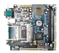
Providing the signature low profile, minimal noise and reduced power of the VIA EPIA series on a 17 by 17cm small form factor, the VIA EPIA MII Mini-ITX Mainboard is an "all-in-one" entertainment platform geared to the digital home. The VIA EPIA MII-Series easily slots in to a digital home infrastructure providing a vast horizon of applications that feature sophisticated connectivity including wired or wireless media servers, mobile PCs, receivers for the living room and beyond.
