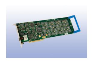
The Diva PRI/E1-30 enables one server to support up to thirty concurrent communications with a mix of ISDN devices, V.90 modems, GSM mobile phones, and fax machines, making it an excellent choice for medium to large businesses. Because it is based on open-systems architecture, most industry-leading fax, unified messaging, computer telephony integration, and Voice over IP (VoIP) applications integrate easily when the Diva PRI/E1-30 is used.
