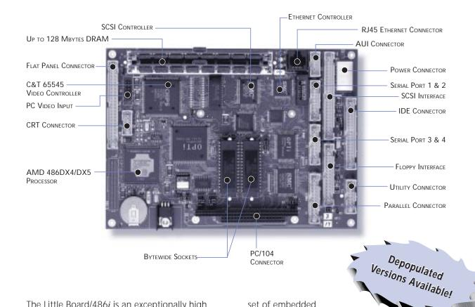
The Little Board/486*i* is an exceptionally high integration, high performance, 486DX-based PC/AT compatible system, in the footprint of a 5-1/4 inch disk drive. This rugged, high quality single-board system contains all the component subsystems of a PC/AT motherboard plus the equivalent of six PC/AT expansion cards.
