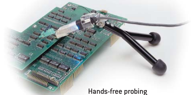
Hands-free probing with FreeHand probe holder and HFP probe
