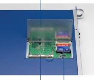
SDRAM socket CompactFlash socket
