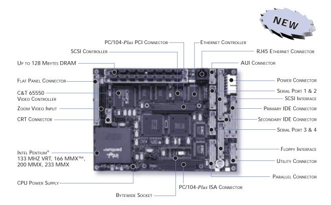
The Little Board/P5*e* sets the standard for Pentiumbased embedded-PC designs. The extreme power of an Intel Pentium processor is combined with the high bandwidth of a PCI expansion bus, in a rugged and reliable single-board solution for embedded applications that demand small size, low power consumption, and high functionality.
