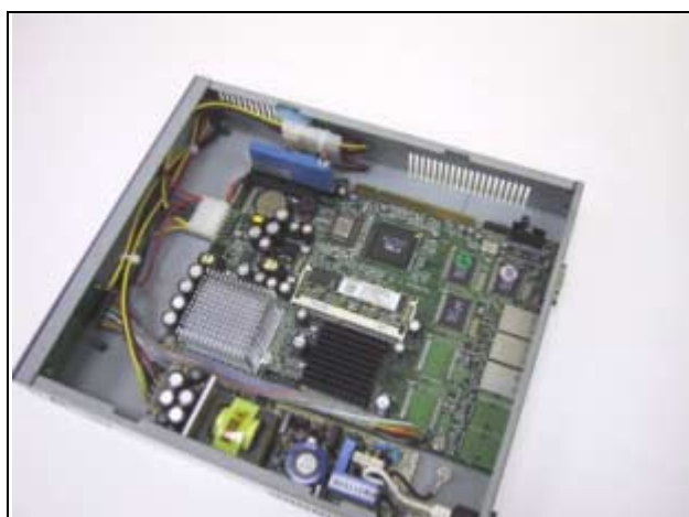
Fig. 2-13 Completion of DOM power connection
