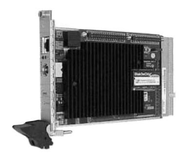
**The cPRO3** 3U System Controller Compact PCI Single Board Computer is an extension of the Proteus family of embedded computers from SBS Technologies. The cPRO3 is targeted for embedded applications and incorporates a Socket 7 processor; offering a variety of high level processor speeds, including Low Power Pentium support. The cPRO3 is based on the CompactPCI (cPCI) specification of the PCI Industrial Computers Manufacturing Group (PICMG).
