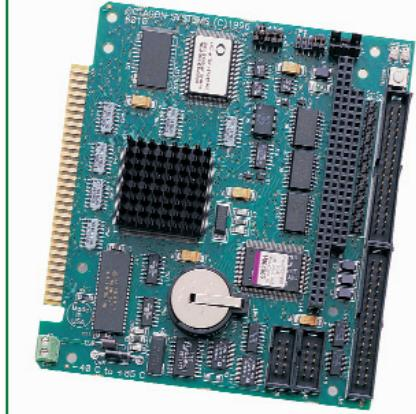
*Octagon products are designed and manufactured under the supervision of an ISO 9001-2000 certified quality management system. The 6010 will withstand high shock and vibration, and operates in temperature ranges from -40° to +85° C. This rugged single board computer will provide years of reliable service in the most challenging environments.*
