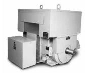
Features: High efficiency (95% or higher), Epoxy ester enamel paint, stainless steel breather drains, ground lug in conduit box, cast iron frame, end shields, DE shaft slinger and shaft cap, ODE shaft cap, epoxy coated rotor OD and stator ID (including windings), lead separator gasket between frame and conduit box. Stock motors include a three year warranty, precision balance, 100 ohm platinum winding RTD's and space heaters.
