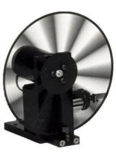
In measurement scenarios where the optical signal to be measured may be confounded with a background optical signal, either from ambient lighting, or, in the infrared, heat (or infrared radiation) emitted by instrumentation and the background, a means of discrimination between the two is required. This is achieved by modulating the desired optical signal on a known carrier wave by an optical chopper.
