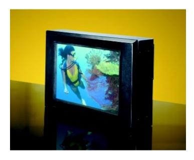
Utilizing our standard enclosure housing design, the EN-C15 offers a 15" XGA AMTFT LCD and three touchscreen choices: resistive, near field imaging and infrared. The system includes up to a 1 GHz Pentium III single board computer with up to 256M of DRAM standard, 10/100BaseT Ethernet, three serial ports and a parallel printer interface. A 2.5" hard drive is integral to the system, and a 3.5" floppy drive is accessible through the side of the enclosure.
