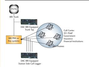
DAC BRIs typically connect to PBXs through a punch-down block at the main distribution frame. The PBX routes calls to to a digital station while the DAC BRI passively taps the line to that station. The DAC BRI can process the data being passed over the line by itself or by handing off the data by MVIP to a separate voice resource card like Ai-logix's SmartDSP VR.
