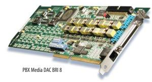
providing a high impedance tap, the DAC BRI 4/8 card has the ability to record both directions of a conversation in a digital format. Designed as an ISA card, and modeled after our industry standard DAC16, it allows call recording developers to easily expand the reach of their call recording solutions with very little effort.
