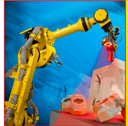
The R-1000iA/80F is equipped with iRVision and other intelligent functions
