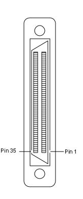
The user interface connections on the SIO4BX is a SCSI II type 68-pin connector (female) mounted to the front edge of the board (P2). The part number for the 68 pin front edge connector is AMP 787170-7. The mating connector is AMP 749111-6 or equivalent. The tables below show the pinout for the RS485/RS422. Single Ended signals (RS-423 and RS-232) use the negative side (-) of the differential pair.
